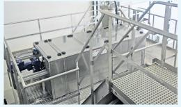
The sludge treatment (MDD-process) has been developed for dewatering and drying of the sludge fraction from effluent treatment in aquaculture. Gas production has been successfully adapted on the basis of sludge, directly from water effluent filtration.
